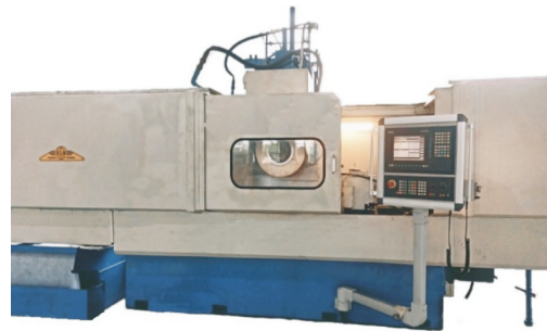
图 2 BC15 缓进磨床 Fig. 2 BC15 creep-feed grinding machine
