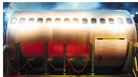
图 6 国产某大型商用飞机铝锂合金机身等直段 Fig. 6 Line part of domestic commercial aircraft's Al-Li alloy fuselage
