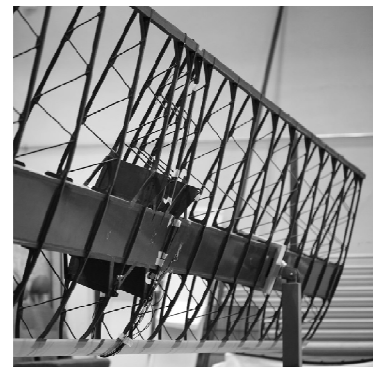
图1 瑞士 Solar Impulse 太阳能飞机翼肋 Fig. 1 Ribs of the Solar Impulse aircraft
