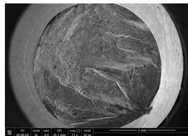
(b) T=25^\circ\text{C} , \sigma_a=500 MPa, N_f=369\,000
