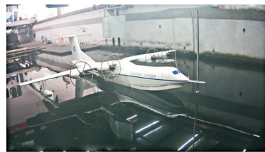
图 1 水池拖曳试验中模型静止时刻的照片 Fig. 1 Photo of the still status of the model in the water tank towing test
