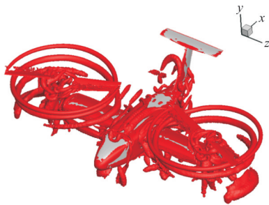
图 6 旋翼/机翼机身间的涡量分布 Fig. 6 Vorticity distribution between rotor and wing
