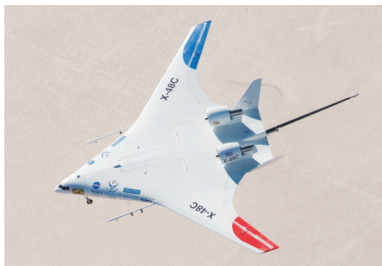
图 7 X-48C 验证机模型飞行试验 Fig. 7 X-48C model aircraft flight test
