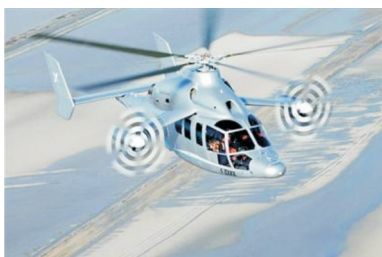
图 1 X3 构型双拉力螺旋桨复合式高速直升机 Fig. 1 Double-thrust-propeller composite high-speed helicopter with X3 configuration
