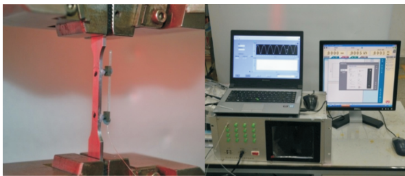
图4 试验机测试件安装及解调系统图 Fig. 4 Installation and demodulation system diagram of test piece of testing machine
