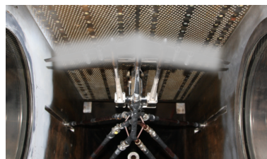
图1 某双体无人机空射平台挂弹CTS试验 Fig. 1 CTS wind tunnel experiment for missile using a double-body airplane as launch platform
