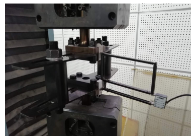
图 8 刚度模拟器测试试验与引伸计的安装 Fig. 8 Stiffness simulator test and extender installation
