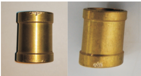
图 13 试验中出现的减压活门磨损情况 Fig. 13 Worn signs of reducer valve during the test
