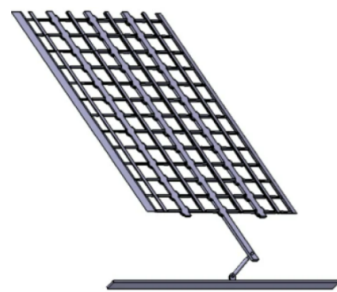
图 14 带剪切蒙皮的变后掠翼 [24] Fig. 14 Variable swept wing with shear skin [24]
