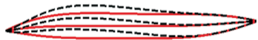
图 20 优化前后机身轮廓变化 Fig. 20 The profile comparison between the basic and optimized fuselage
