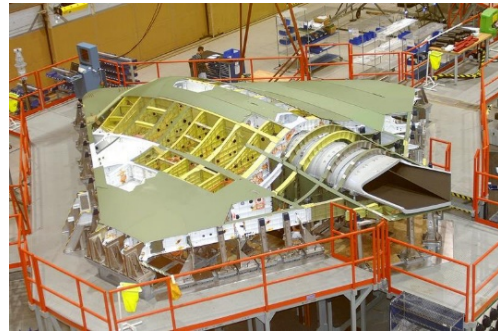
图 6 飞翼机体与进排气系统的融合示例(X-47B) [4] Fig. 6 An illustration of airframe integrated with intake and exhaust for flying wing (X-47B) [4]
