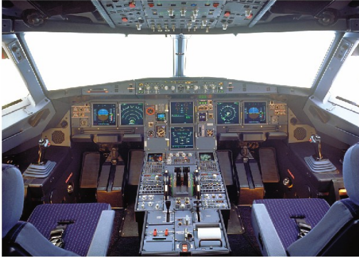
图 2 A320 驾驶舱——典型玻璃座舱驾驶舱 [4] Fig. 2 A320 cockpit: typical glass cockpit [4]
