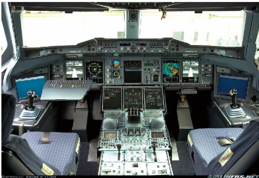
图 3 A380 驾驶舱——典型彩色液晶显示驾驶舱 [4] Fig. 3 A380 cockpit: typical color liquid crystal display cockpit [4]
