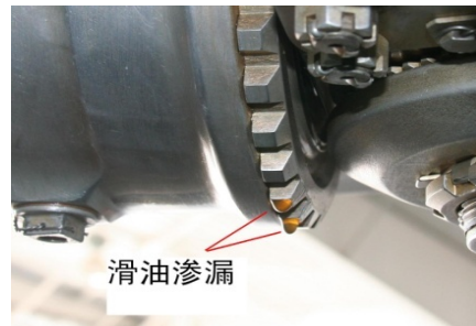
图14 旋翼关节轴承磨损 Fig. 14 Rotor joint bearing wear
