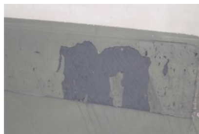
图10 沙尘冲击导致桨叶下表面防护漆层脱落 Fig. 10 Sand impact causes the protective paint layer on the lower surface of the blade to fall off.
