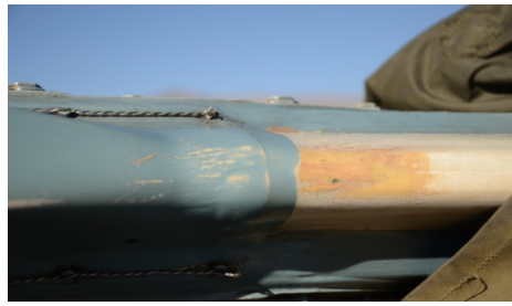
图13 旋翼磨损、涂层剥落 Fig. 13 Rotor wear and coating peeling
