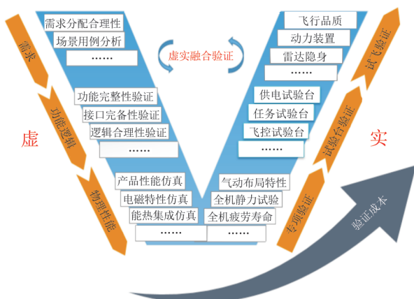
图9 面向试验的复杂系统虚拟验证技术 Fig. 9 Testing-oriented complex system virtual verification technology
